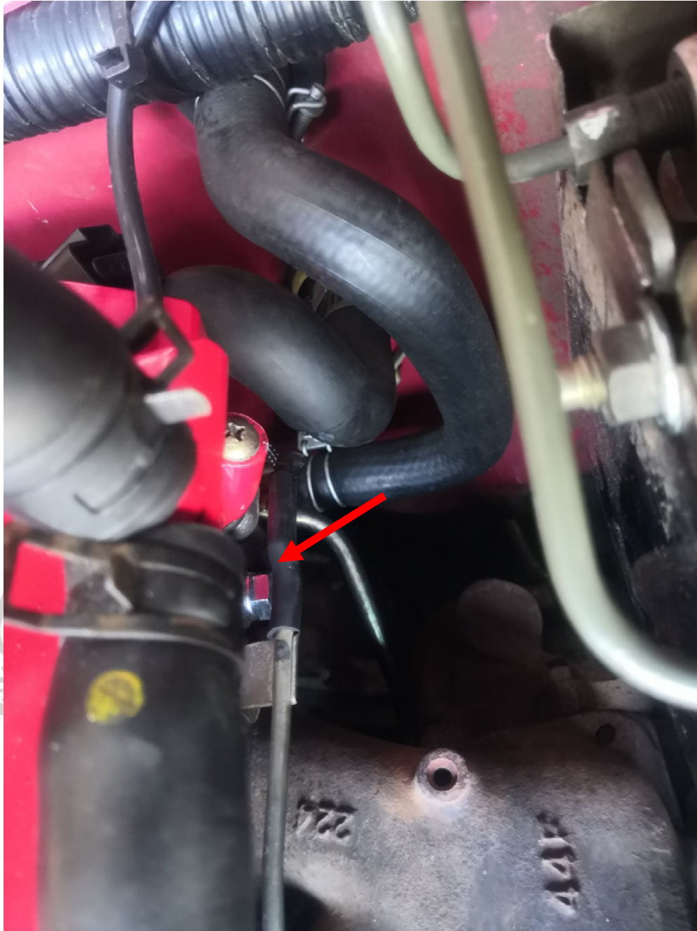
Figure 6 – Bolt Down the Other Ground Wire Ring on the Engine Lift Point (Exhaust Side) Using the Supplied Bolt
