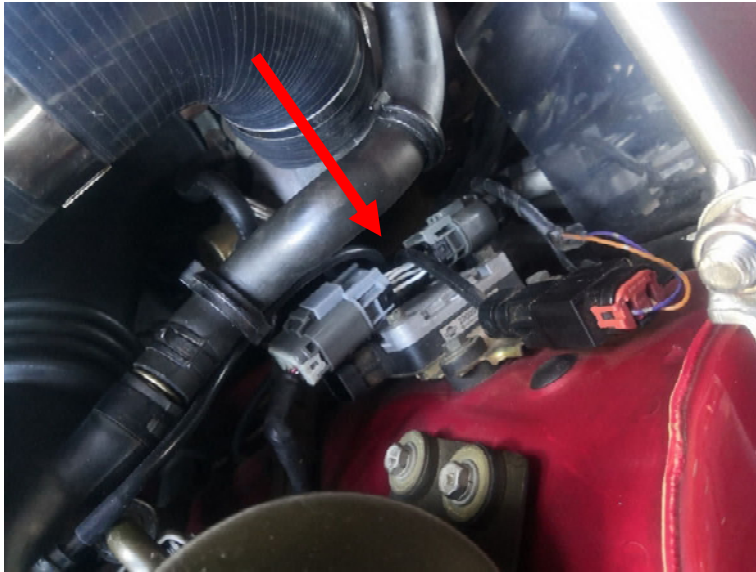
Figure 7 - Connect Igniter Patch Harness (Exhaust Side Strut Tower). Remove the Old Igniter If Necessary
